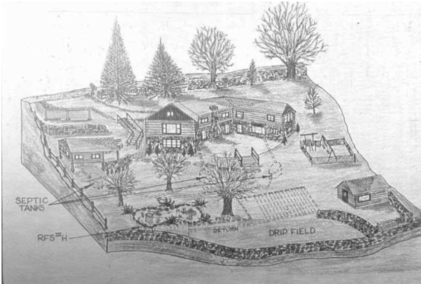
Figure 1.2 Architectural concept drawing of advanced onsite wastewater system technology (RFS III H and Drip) for a single family built on a lake front property. (Courtesy of ASHCO-A-Corporation, Morgantown, WV)
